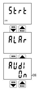
First selection is START/STOP logging. There are two possibilities: if logging is stopped, logging start is offered (symbol Strt = START), if logging is in progress already, logging stop is offered (reading STOP). Press ENTER key to confirm one of two possibilities. Notice: if battery voltage is low it is not possible to start logging.
